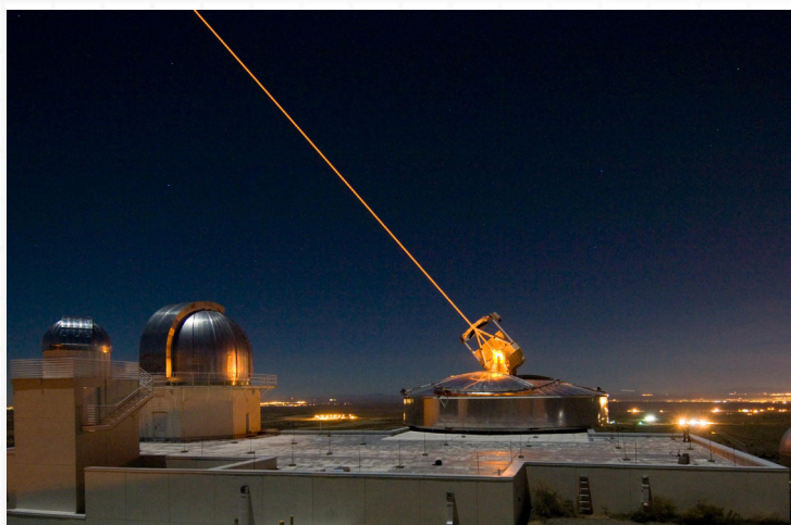
The sodium laser excites sodium atoms in the upper atmosphere to create a source of light or beacon 90 kilometers (55 miles) above the Earth. The adaptive optics system measures distortions of this beacon caused by atmospheric turbulence. The system then sends signals to actuators that alter the shape of a thin mirror thousands of times per second to compensate for atmospheric distortion of the image. (Photo/AFRL)
