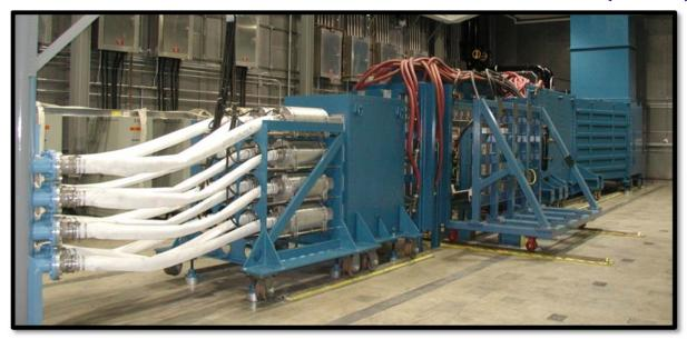
**Purpose:** The CEAC imposes combined acoustic, thermal, and mechanical loads on aerospace structures. The CEAC is employed to measure structural response and determine acoustic fatigue life of structural components when exposed to simulated aeroacoustic and thermal loads. The CEAC is used to validate advanced technologies for hypersonic, space access, weapons bay, and exhaust-washed vehicle structures.
