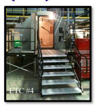
**Purpose:** The ETCs test the structural integrity of aerospace structures in representative operating temperatures and aerodynamic load distributions. The test article may be tested in an inert atmosphere. The ETCs are utilized to validate design and analysis of advanced structures technology for extreme thermal and mechanical applications such as hypersonic structures and thermal protection systems.
