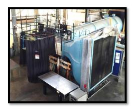
produce controllable turbulence levels of up to 15%. In addition a moving bar wake generator is available to introduce unsteady periodic upstream wakes at reduced frequencies typical of engine operations. The inlet and test sections pivot with respect to the fixed exit section, allowing the cascade inlet and exit angles to be set independently between 0° and 65°, accommodating a total
