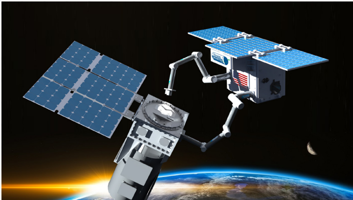
A concept for a generalized two-arm servicer for satellite repair and refuel (Photo by Tethers Unlimited)
