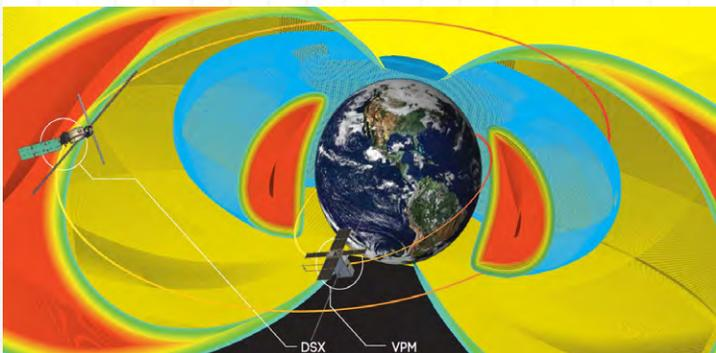
VPM's orbit with respect to DSX's orbit. The rings are the various L-shells comprising the Earth's magnetic fields within the magnetosphere.
