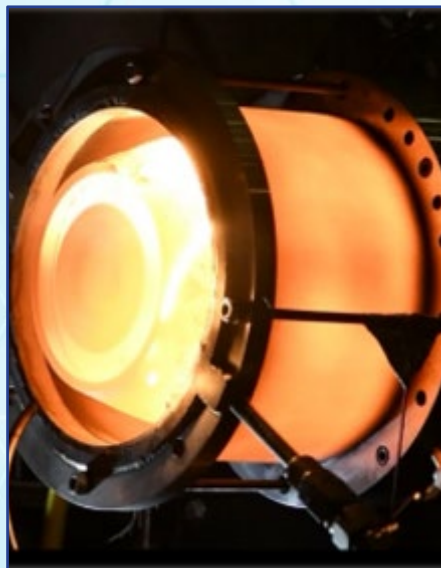
Ceramics Parts in Rotary Detonation Engine Test
