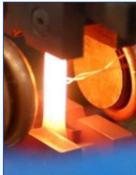
Micro-Testing of a High Temperature Metal With Side Induction Heating
